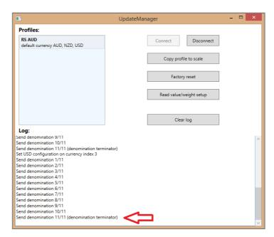
**8.** Click on [ Disconnect ] to finish the connection between the scale and the PC and unplug the USB cable from the back of the scale..
